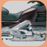
Powerful 1,832cm<sup>3</sup> liquid-cooled horizontally-opposed six-cylinder engine with PGM-FI fuel injection system features all-new Linear Air/Fuel (LAF) low emissions system, which more accurately controls both carburetion and emissions for unprecedented reductions in harmful emissions. Measured output is less than half the limits imposed by strict new EURO-3 regulations.
